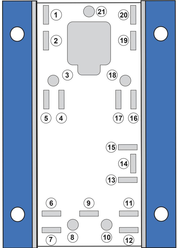
1. **PORT REGULATOR FIELD INPUT TERMINAL** - Connect Terminal #1 to port voltage regulator's Field Output terminal via a user-supplied 12-gauge BLUE wire. A female 1/4" spade terminal is supplied for connection to Terminal #1. The 12-gauge BLUE wire will replace the regulator's 14-gauge field wire.
