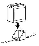
Insert a new, full, and sealed original EFOY fuel cartridge into the fuel cartridge holder.
