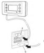
Disconnect the charge line (2) and data line (1) for the operating panel from the EFOY COMFORT fuel cell.
