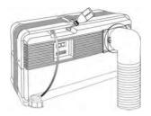
Insert the tip of the bottle into the connection nozzle on the device and slowly squeeze the entire contents into the opening.
