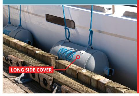
All cylindrical fender models <u>C84</u> and larger must use the <u>Long Side</u> <u>Cover</u> when hung horizontally.
