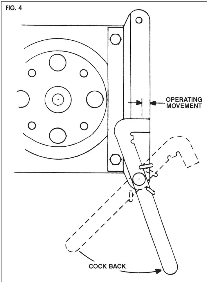
4. Cock locking handle back as illustrated in Fig. 4. Now, tighten nut (G) as shown in Fig. 3.
