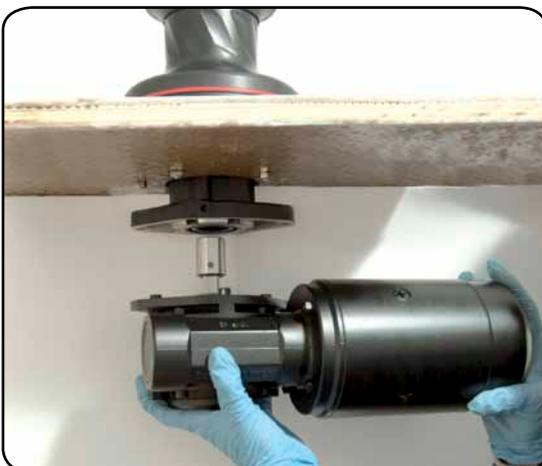
3. Position the reduction gear and motor
