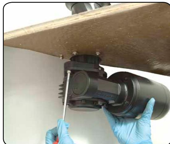
4. Tighten the two screws (8 Nm/ 70in-lb). Be sure to align the flange.
