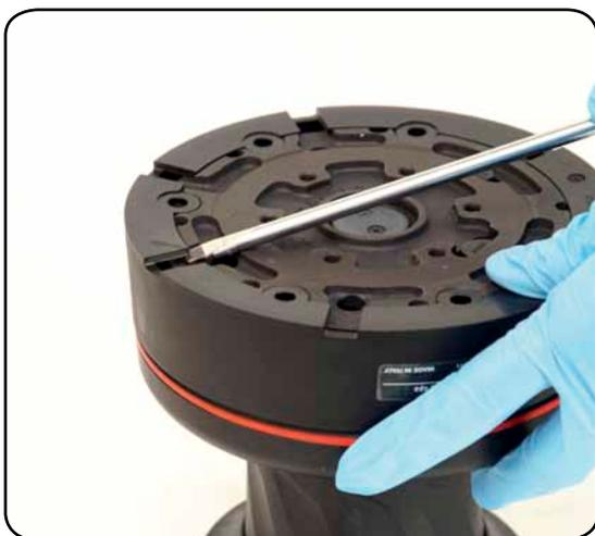
1. Remove the skirt n°2 with the help of the screwdriver placed as shown by the symbol
