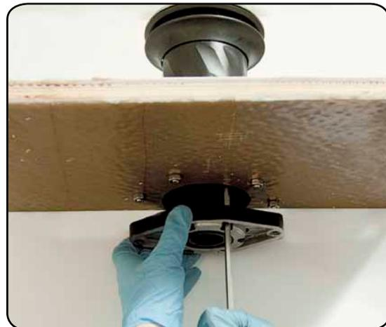
2. Tighten six M6 precote coated screws (8 Nm/ 70 in-lb)
