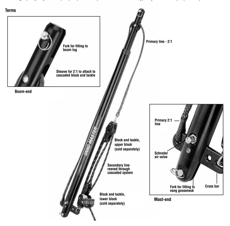
Vang-Master rigid vangs are available for boats with vang fittings on the boom and mast partner. If your boat is not equipped with vang fittings on mast and boom, or if fitting width or pin diameter will not fit jaw and pin sizes listed in the chart below, contact Harken for information.
