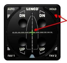
ONCE THE AUTO GLIDE HAS SAVED THE ALTERNATIVE HOME ROLL AND PITCH POSITIONS FOR "HOLD", THE LED INDICATOR WILL ILLUMINATE.
