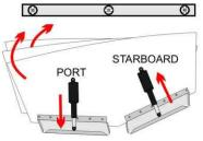
THE STARBOARD TRIM TAB IS MOVED UP AND THE PORT TRIM TAB IS MOVED DOWN IN SHORT, EQUAL BURSTS UNTIL THE BOAT'S CURRENT ROLL POSITION MATCHES THE AUTO GLIDE'S HOME ROLL DEFAULT POSITION
