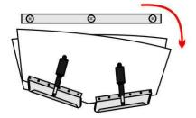
You must find your desired roll and pitch position by manually operating the trim tabs. Once the boat reaches the desired roll and pitch angles, press and hold the <u>"FAV 1" or "FAV 2" BUTTON</u> until the corresponding <u>"FAV 1" or "FAV 2" LED INDICATOR</u> flashes five (5) times. Once the <u>"FAV 1" or "FAV 2" LED INDICATOR</u> stops flashing, the Auto Glide saves the alternative <u>HOME ROLL AND PITCH POSITION</u> and the boat will begin leveling around that roll and pitch angle.
