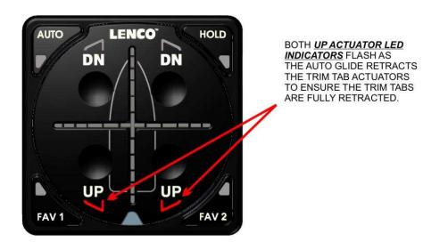
Once the Auto Glide "wakes up", it takes a few moments to verify that it is receiving all of the required ENGINE and GPS DATA and that both <u>HOME ROLL AND PITCH DEFAULT POSITIONS</u> have been stored. It then defaults to the "<u>AUTO" AUTOMATIC SETTING</u> and <u>IDLE MODE.</u>
