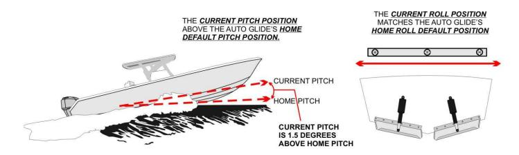
THE 3RD LED ON THE BOTTOM HALF OF THE VERTICAL CROSSHAIR LED INDICATOR IS ILLUMINATED TO INDICATE THAT THE BOAT'S **CURRENT PITCH POSITION** IS ABOVE THE AUTO GLIDE'S **HOME PITCH DEFAULT POSITION**.
