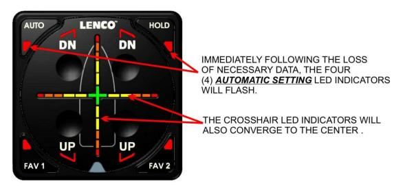
As soon as the initial LED flash sequence is over, the Key Pad will begin to flash a **SYSTEM FAILURE**WARNING MESSAGE and begin to automatically retract the trim tabs in short bursts until they are fully retracted.
