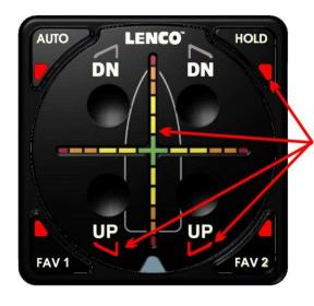
DEPENDING ON THE TYPE OF DATA LOSS, THE AUTO GLIDE WILL FLASH A SEQUENCE OF **SYSTEM FAILURE WARNING MESSAGES**.
