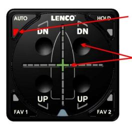
WHEN THE "AUTO" LED INDICATOR IS ILLUMINATED, THE AUTO GLIDE USES THE HOME ROLL AND PITCH DEFAULT POSITIONS THAT WERE SAVED DURING THE AUTO GLIDE SETUP PROCESS DESCRIBED IN OWNER"S MANUAL A.
