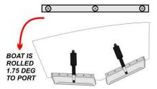
THE 2ND LED ON THE PORT SIDE OF THE HORIZONTAL CROSSHAIR LED INDICATOR IS ILLUMINATED TO INDICATE THAT THE BOAT'S CURRENT ROLL POSITION IS ROLLED TO THE PORT OF THE AUTO GLIDE'S HOME ROLL DEFAULT POSITION.
