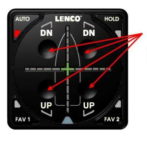
PRESS ANY OF THE FOUR (4) UP/DN BUTTONS TO ACTIVATE **MANUAL MODE.**
