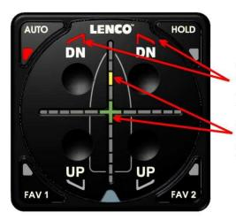
AS SOON AS THE AUTO GLIDE ENTERS INTO HOLE SHOT MODE, IT FULLY DEPLOYS THE TRIM TABS UNLESS THE SEA CONDITIONS ARE TOO ROUGH. ROUGH WATER HOLE SHOT IS COVERED ON PAGE 12.
