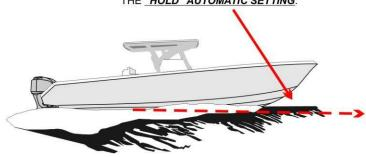
THE STARBOARD ROLL ANGLE WILL ALSO BECOME THE TEMPORARY HOME ROLL POSITION FOR THE "HOLD" AUTOMATIC SETTING..
