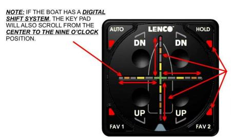
IF THE LOST GPS OR ENGINE DATA IS REACQUIRED BY THE AUTO GLIDE, IT WILL FLASH THE OUTSIDE FOUR (4) AUTOMATIC SETTING LED INDICATORS AND ALL FOUR (4) QUADRANTS OF THE CROSSHAIR LED INDICATORS.
