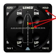
ONCE THE BOAT HAS REACHED THE DESIRED PITCH AND ROLL ANGLE, <u>PRESS AND RELEASE</u> THE <u>"HOLD"</u> BUTTON.
