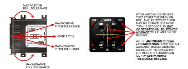
Once the Auto Glide defaults to <u>LIMP HOME MODE</u> and displays an <u>OUT OF OPERATIONAL TOLERANCE</u> <u>FAILURE MESSAGE</u>, you will have to verify the Auto Glide Control Box is installed properly (See Section 2.3 in Owner's Manual A) and then reset the Auto Glide by turning your motor(s) "OFF" then "ON" again.
