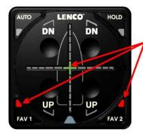
ONCE THE AUTO GLIDE HAS SAVED THE ALTERNATIVE HOME ROLL AND PITCH POSITIONS FOR "FAV 1" OR "FAV 2", THE CORRESPONDING LED INDICATOR WILL FLASH FIVE (5) TIMES.
