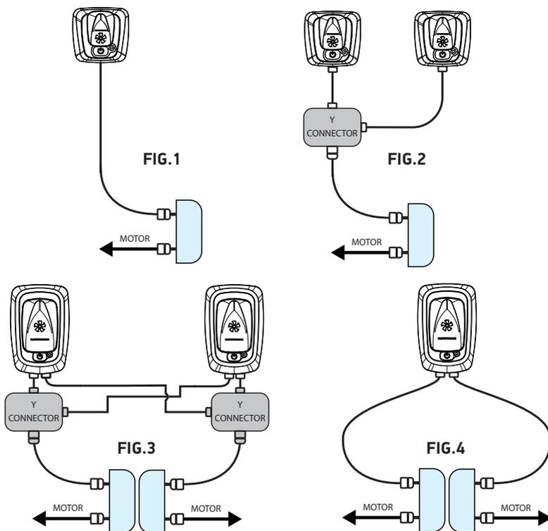
The legacy converter is required to be able to use a new style (gen2) control panel with an old style (gen1) thruster.
