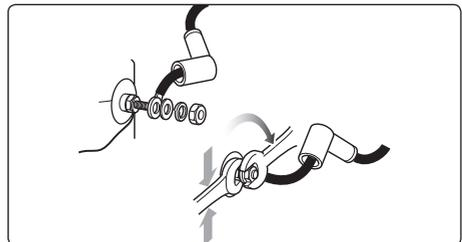
DO NOT overtighten electric motor terminal nuts.
