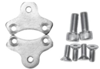
**ADAPTER MOUNTING KIT:** Enables the installation of a split ring anode onto the lower units of Yanmar SD20, SD30, SD31, SD40, SD50 and SD60 saildrives. Contains: 2 x Stainless Steel Plates, 4 x Screw DIN7991 (countersink w/hex socket head) M6 x 1.0 - 16, 2 x Screw DIN912 (Hex Socket Head) M8 x 1.25 - 20
