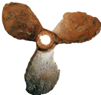
On wood and GRP vessels the areas of concern are principally the stern gear i.e. The propellers, shafts, shaft brackets, stern tubes and rudders which are expensive to replace and vital to the vessel, the failure of a propeller or rudder could have disastrous consequences. The effects of corrosion can vary from pitting of propellers and shafts to the decomposition of the alloy of propeller. The failure of something as small and inexpensive as a split pin can result in the loss of the propeller.
