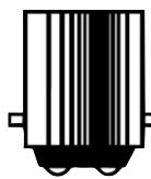
**Fig. 0337****Fig. 0375 - Double Contact Bayonet Indexing Base Bulb**
