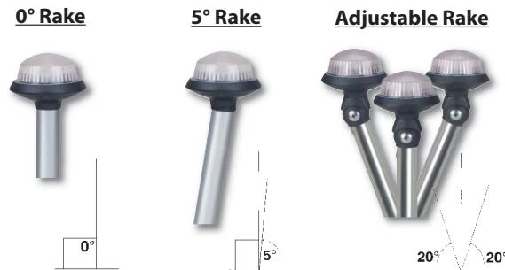
Rake is determined by the pole, base and base location angles. Rake is important for all reduced glare lights to insure that light output is correct. The most common rake angles are 0°, 5° and 16°. Custom made poles often have non-standard rake angles. Choose from 0°, 5° or fully adjustable versions (Delta, Stealth and Omega Series).
