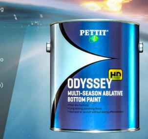
**APPLICATION SYSTEMS:** Odyssey HD is easily applied by brush, roller or spray. When rolling use only a high-quality roller cover. Odyssey HD can be applied with a 3/8" roller. For a smoother finish, Odyssey HD can be applied with a short nap 1/4" roller or thin Odyssey HD with Pettit 120 Brushing Thinner 10%
