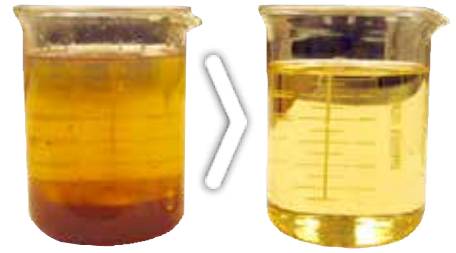
Photo shows unfiltered diesel fuel on the left, filtered diesel on the right.
