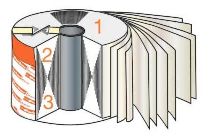
Racor Absolute is a unique oil cleaning system that puts theoretical filtration principles and mechanisms into practice. Low flow, low pressure, and axial filtration combined with special cellulose filter material enables us to achieve ultimate filtration.
