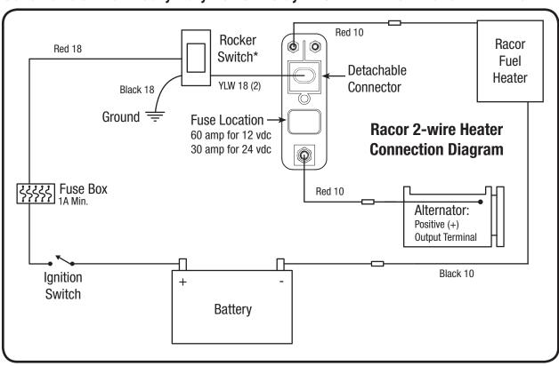
Schematic D - For Heavy-Duty Power Relay Kits: RK 19490-12 and RK 19490-24
