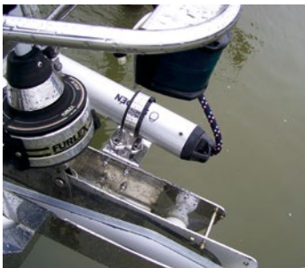
Side mounted installation on stem head anchor fitting.
