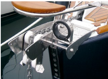
Bow bracket integrated with bow anchor fitting.
