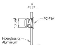
PC-F1A can be used as screw / friction fit into thin frames & seat backs
