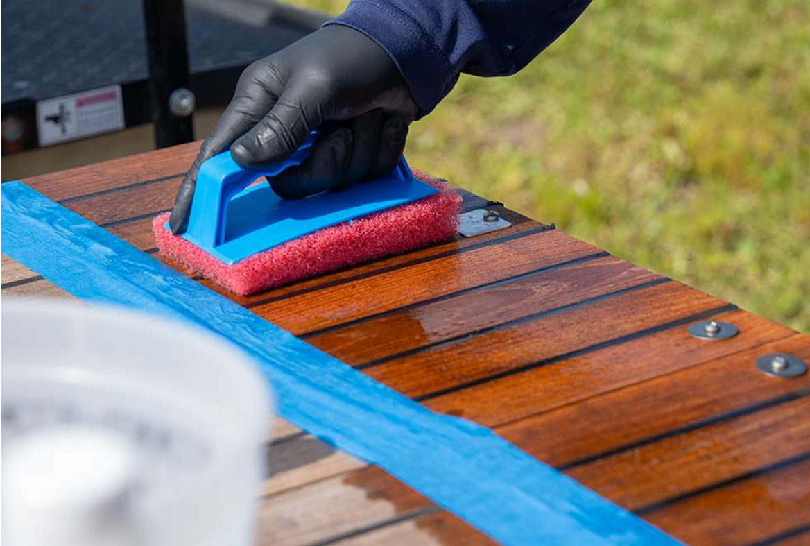
Apply to Deck: Simply Pour On and spread evenly with Brush or Squeegee, then Wait 2-5minutes and do not allow the mixture to Dry, also keep moist by reapplying the mixture as needed.
