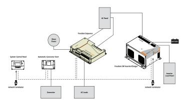
Figure 2 Typical Xanbus System Diagram
