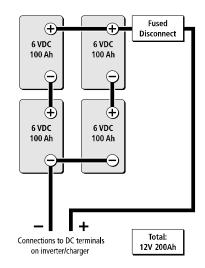
Figure 25 Batteries in Series-Parallel Connections
