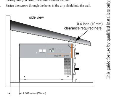
Figure 26 Drip Shield Placement (Desktop Mount)
