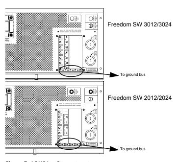
Figure 7 AC Wiring Compartment
