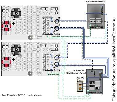
Figure 17 Parallel Stacking Using Two Freedom SW 3012s
