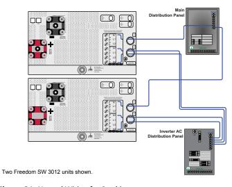
Figure 21 Neutral Wiring for Stacking
