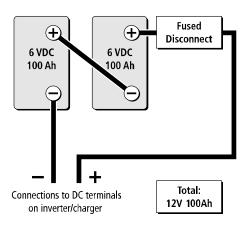
Figure 24 Batteries Connected in Series
