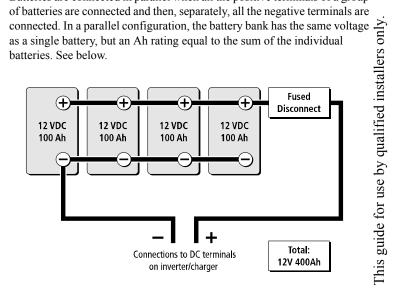
Figure 23 Batteries Connected in Parallel
