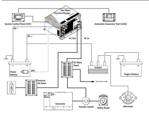
**IMPORTANT:** Figure 3 does not show all required grounding or overcurrent protection. See the next two pages as well as on page 17 for required DC grounding or overcurrent protection.
